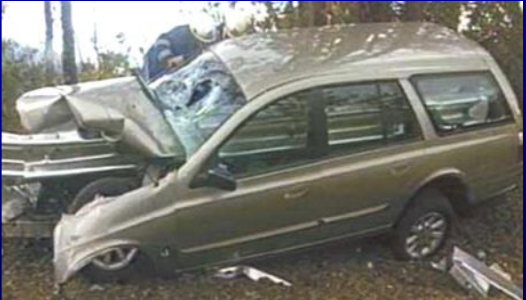
Blunt guardrail end treatment
